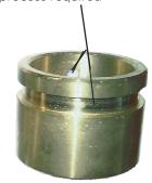
Dove tail in bushing. Packing gland holds bushing in place. Used to pull bushing from pump bushing from pump
