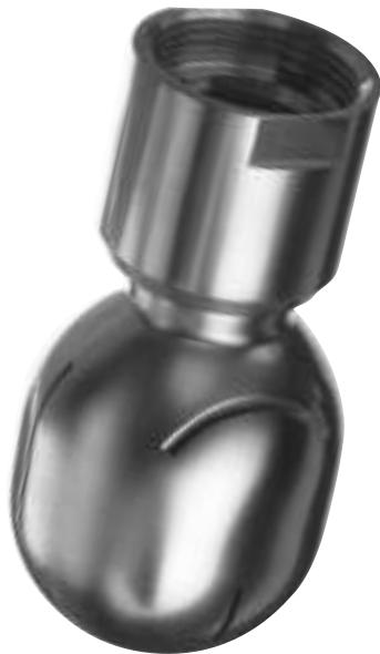
The Maxi rotary spray head provides a rotating fan cleaning action using low volumes of liquid at low pressure. It is an automatic device for cleaning medium size tanks and a more efficient replacement for traditional fixed sprayballs or manual methods used in tank cleaning.
