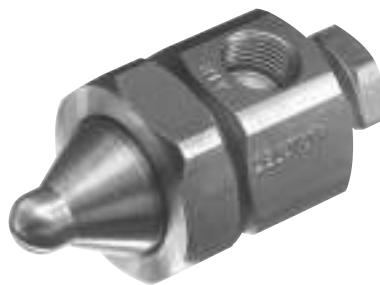
The AL 60 series produces a wide angle flat fan spray pattern with a nominal angle of 90°-110°. This is an internal mix nozzle, where a change in air or liquid pressure will result in a change of flow or atomisation. Increasing air pressure decreases flow and increases atomisation. Increasing liquid pressure increases flow and decreases atomisation.
