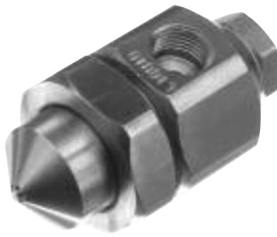
The AL 30 series produces a wide, round spray pattern with a nominal angle of 70°. This is an internal mix nozzle, where a change in air or liquid pressure will result in a change of flow or atomisation. Increasing air pressure decreases flow and increases atomisation. Increasing liquid pressure increases flow and decreases atomisation.
