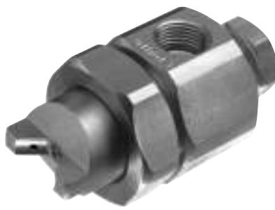
The AL 15 series is a pressure-fed external mix flat fan spray nozzle. The external mix feature allows control of the atomisation without changing liquid flow. The lighter the air pressure, the higher the atomisation for a given liquid pressure (types 15-06 to 15-11). Types 15-01 to 15-05 are siphon type. The spray pattern is a function of pressure. The higher the air pressure, the longer the spray pattern (length D).
