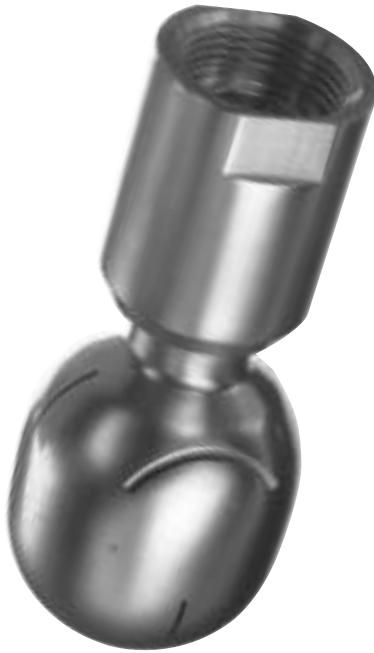
The Mini rotary spray head provides a rotating fan cleaning action using low volumes of liquid at low pressure. It is an automatic device for cleaning small tanks and represents a more efficient replacement for traditional fixed sprayballs or manual methods used in tank cleaning.
